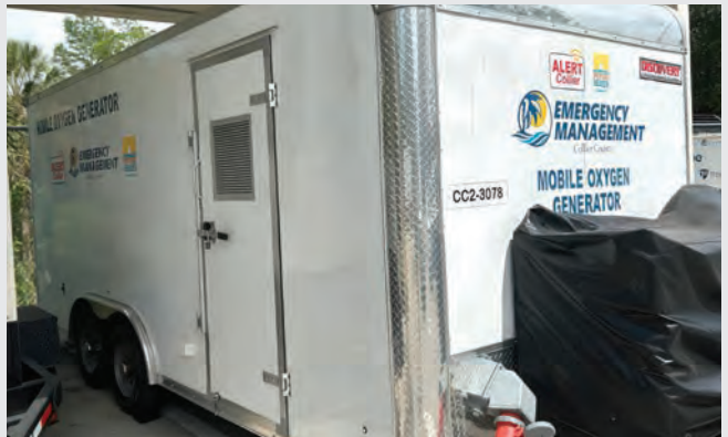
▲ Collier County, Florida, has a mobile medical oxygen generator system so residents who use oxygen devices can refill their tank during power outages.
